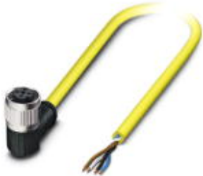
Sensor/Actuator cable, 4-position, PVC, Yellow RAL 1021, Free cable end, on Socket angled M12-SPEEDCON, A-coded, Cable length: 2 m
